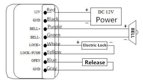
Remark: Jumper Cap on NC terminal for Power Off unlocking and NO terminal for Power ON unlocking (in this case please set Unlocking Duration to be [00]).
